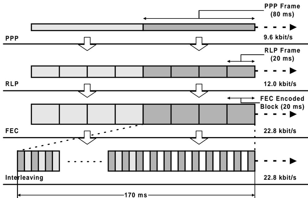
**Figure 2-9:** Error control in GSM Circuit-Switched Data.
